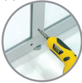
Connect middle rail(s)\* to the bottom rail and tighten grub screws. The middle rails have a double graphic fitting strip on them. They will balance.
