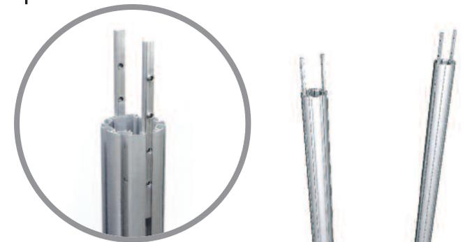
Stand base on the ground. Loosen grub screws and slide both connector bars half way out of groove and retighten. Repeat for other base post.
