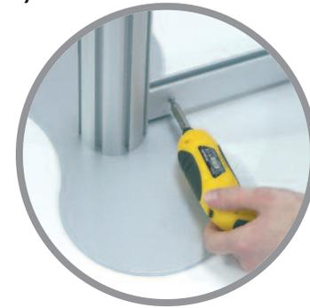
Connect the bottom horizontal rail to the two posts and tighten grub screws as before. Leave top rail until all verticals are in place. They will balance.
